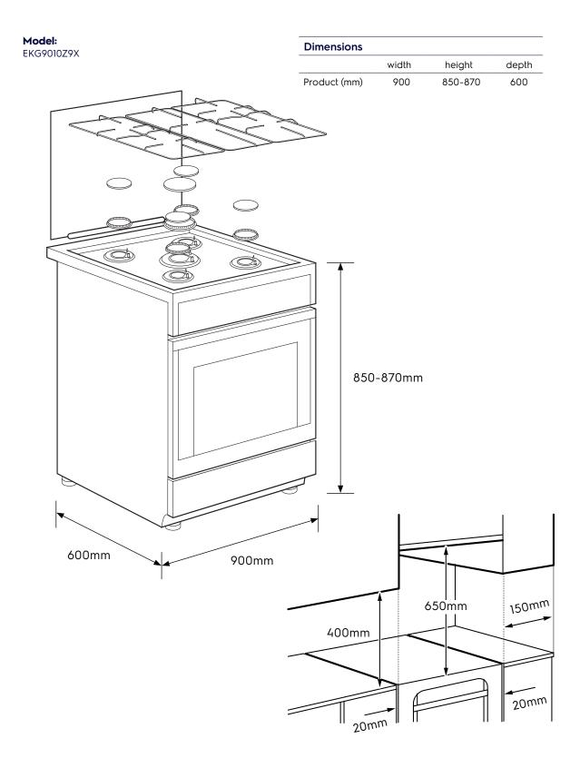
Please note! Dimensions to be used as a guide only. All customers MUST refer to the user manual supplied with the product for detailed installation instructions. © 2023 Electrolux S.E.A PTE. LTD. E\_DIM\_EKG9010Z9X\_Jan23
