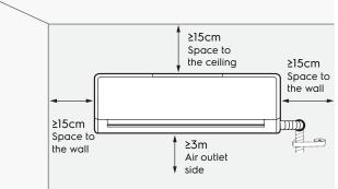
Please note! Dimensions to be used as a guide only. All customers MUST refer to the user manual supplied with the product for detailed installation instructions. © 2022 Electrolux S.E.A PTE. LTD. E\_DIM\_ESF303C1WAI\_Jan22
