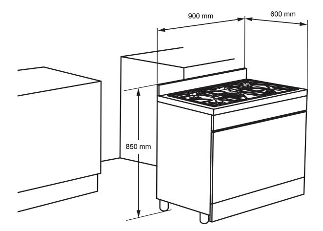
Please note! Dimensions to be used as a guide only. All customers MUST refer to the user manual supplied with the product for detailed installation instructions. © 2021 Electrolux S.E.A PTE.LTD. EKG9241Z7X\_Dim\_Aug21
