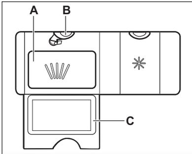
1. Press the release button (B) to open the lid (C).
